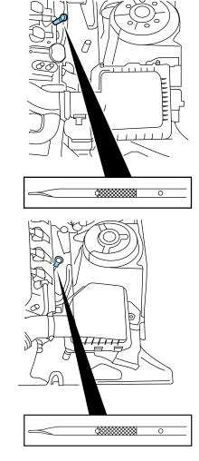
• 5.0L V8 engine - Locate the engine oil dipstick by reaching between the strut tower brace (if equipped) and the hood hinge area.
